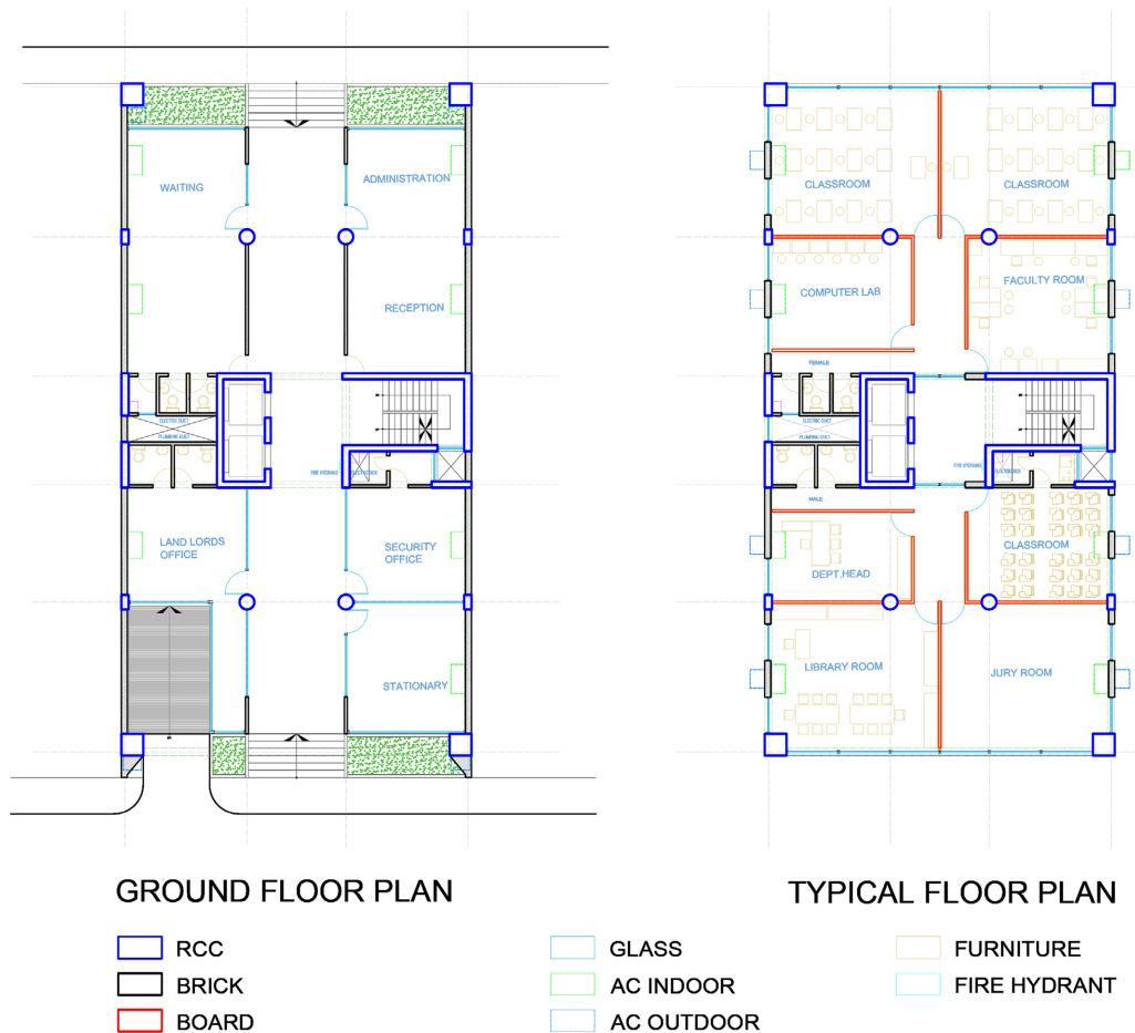
Figure 10. Plans of star tower.
