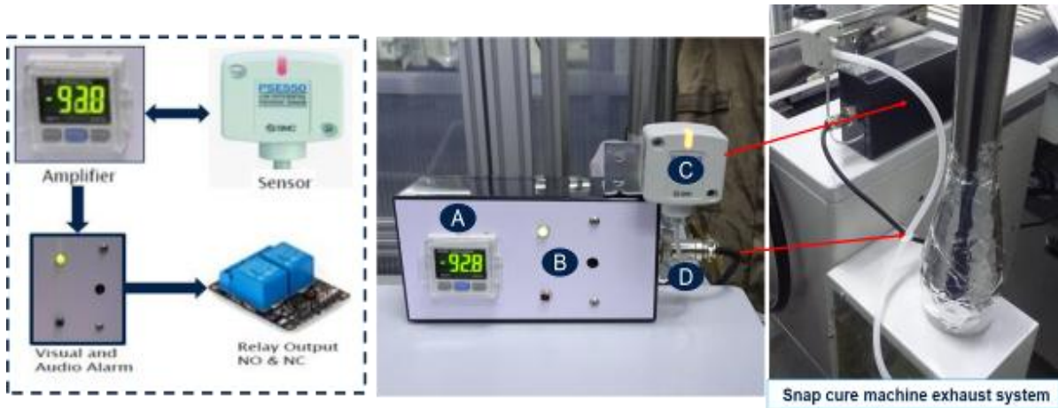
Fig. 5. Digital exhaust controller
