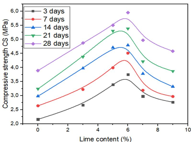
Fig. 7. Changes in compressive strength as a function of lime content
