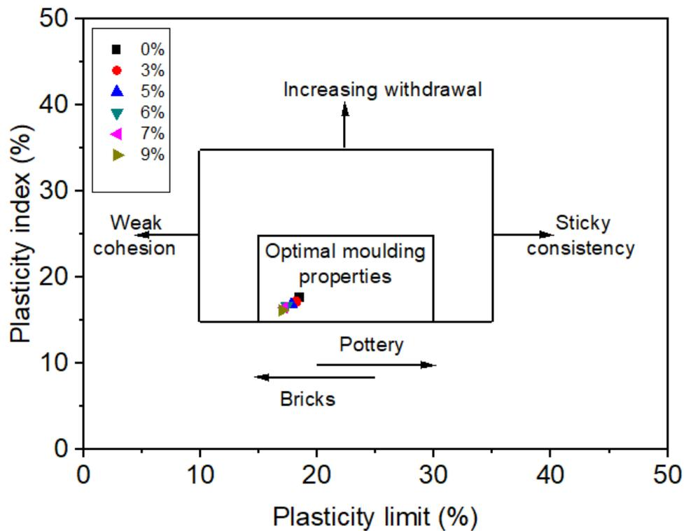
Fig. 4. Casagrande plasticity diagram showing the moulding properties of soils as a function of their Atterberg limit
