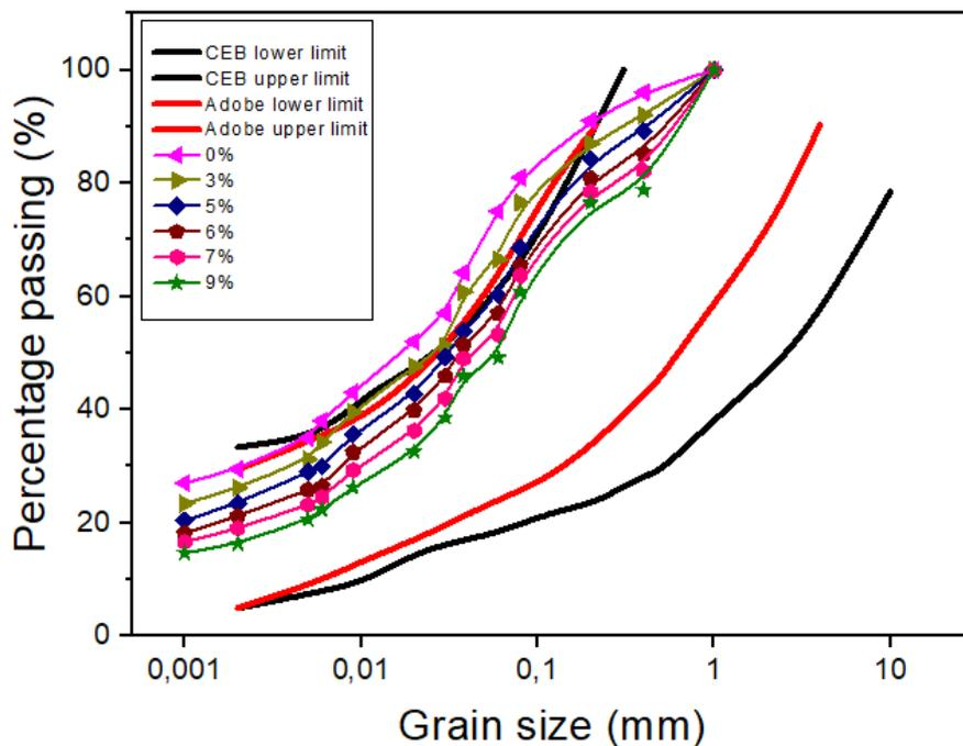
**Fig. 2. Sieve size curves for raw soil and mixes with 3%, 5%, 6%, 7% and 9% lime, based on the normative ranges for Adobes and compressed earth bricks (CEB) [19]**
