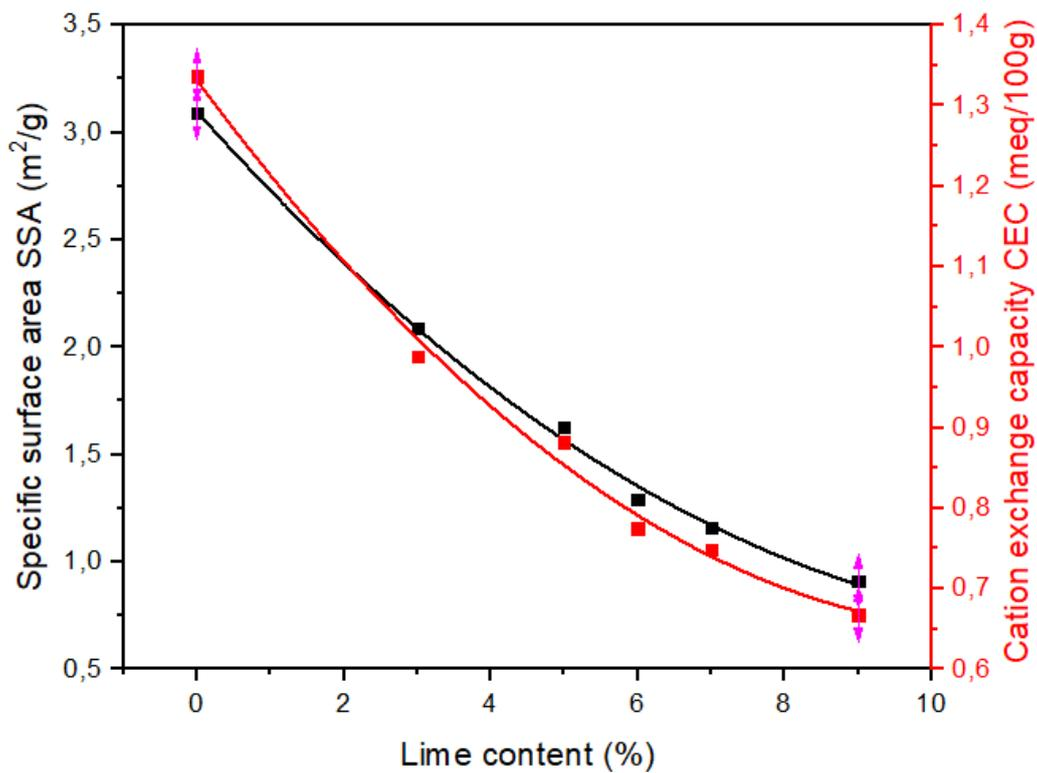
Fig. 6. Changes in the specific surface area and cation exchange capacity of soil as a function of lime content
