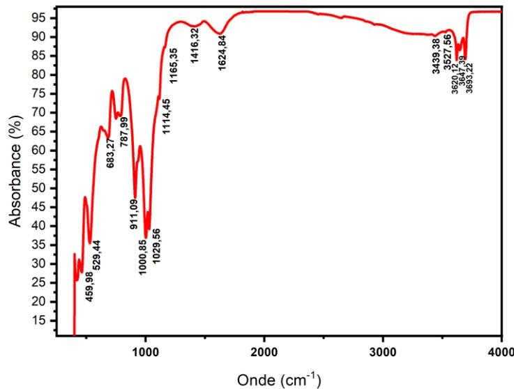
Fig. 8. Infrared spectrum of the cubitermes sp termite mound soil
