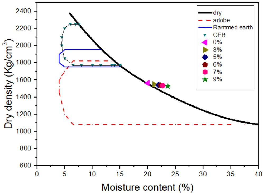
Fig. 5. Dry density based on optimum soil moisture content and recommended surfaces for CEB, Rammed earth and Adobe according to Delgado M.C.J., Guerrero I.C. 2007 [19].
