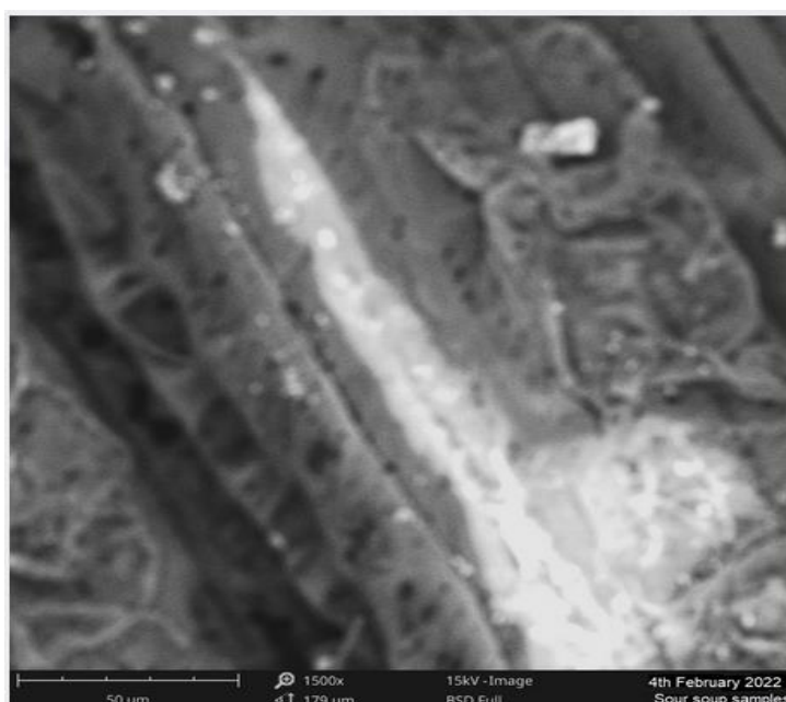
Fig. 4. Scanning electron microphotograph of the biosynthesized silver nanoparticle (1500x magnification)
