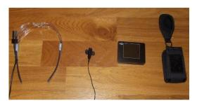
Fig. 1. SEBE equipment for NPP workers: Subcam on glasses, microphone, camcorder and bag
