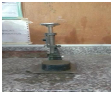
Fig. 1. Vicat apparatus test setup for setting times
