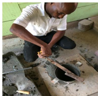
Fig. 2. Laboratory investigation of workability test on concrete
