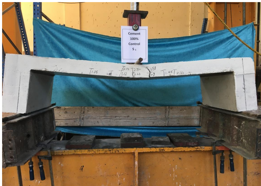
Fig. 2. Test setup and slabs under testing
