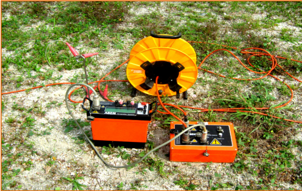
Figure 9. Viewing the instrument type SAS1000 applied in geophysical survey technique
