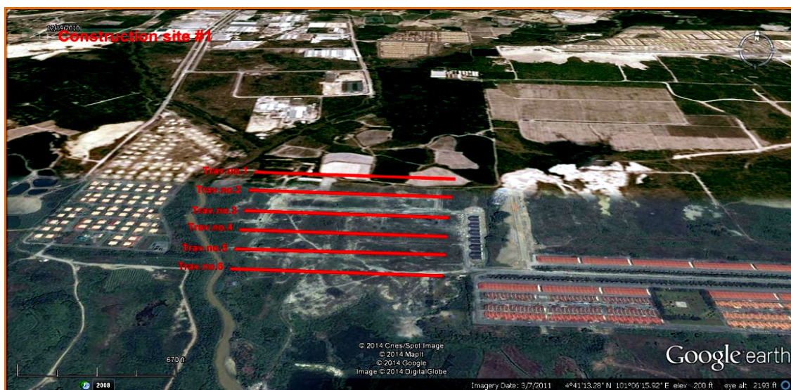
Figure 10. Google earth satellite images (2011) viewing the location of resistivity profiles in construction site #1
