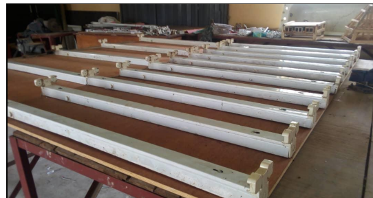
Fig. 1. Arrangement of as-built lamps for pre-retrofits data collection
