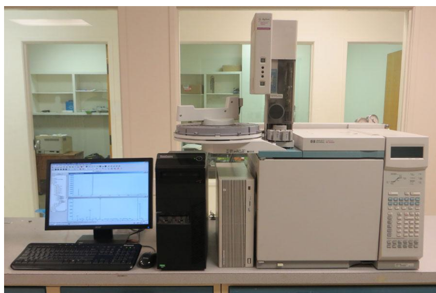
Plate 9. The gas chromatography system used
