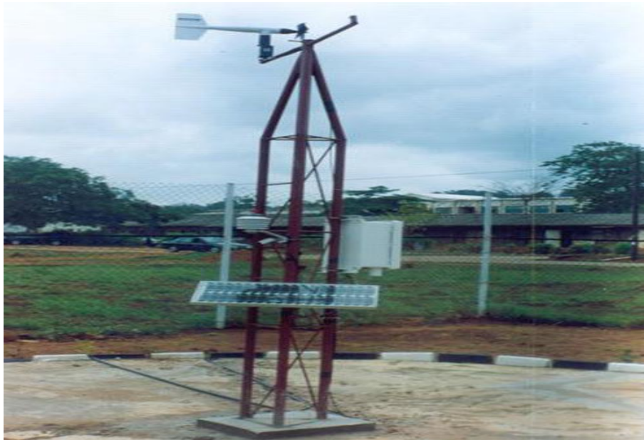
Fig. 2. Tropospheric data acquisition network (TRODAN) set up at a location
